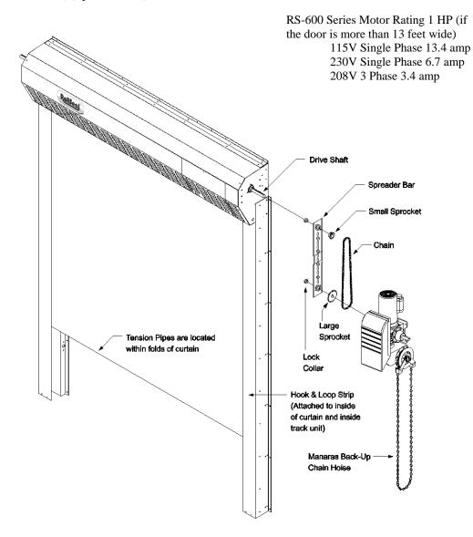
NOTE: Manaras GH Operator can be mounted in its normal upright position for all options. However it may be necessary to remove and re-install the chain and pulley on the opposite side to prevent chain interference. Refer to Manaras Opera GH Installation & Instruction Manual if your operator is a gear head operator.
