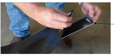
Re-install the "new" floating. It may be necessary to bend one end of the PIM plate up to attach onto the end PIM bolt.
