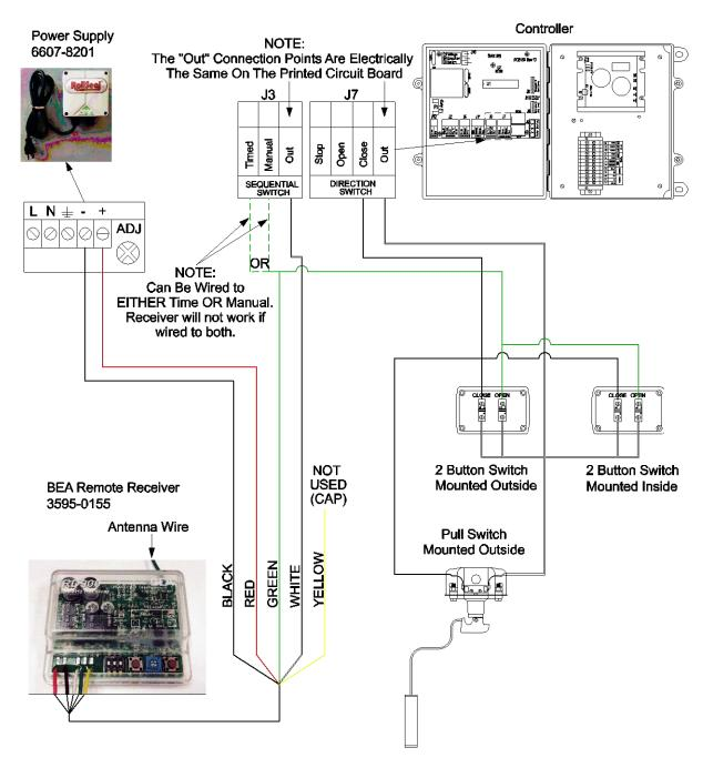
NOTE: Use 18 Gauge Wire for Switches and Seal All Open Areas With Silicone
