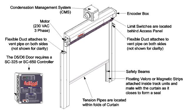
Note: Impact Resistant Pipes are available for door sizes up to 12 feet Soft Tension Pipes are available for door sizes up to 10 feet
