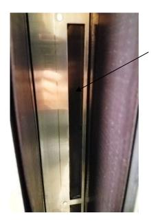
CMS EQUIPPED UNITS ONLY. Cut out floating fabric where slots are located in the PIM plate to allow for air movement.
