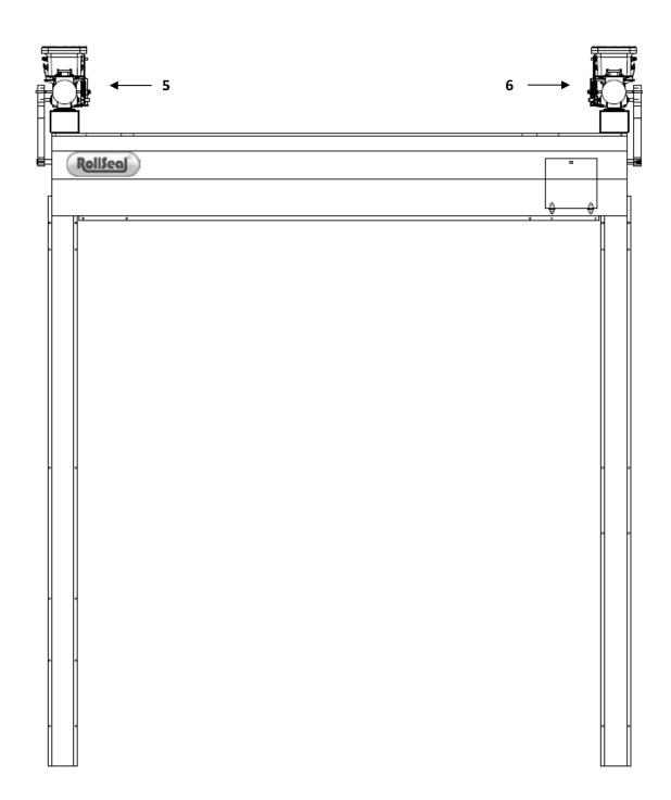
**POSITION 1** – GH motor mounted on the left side.
