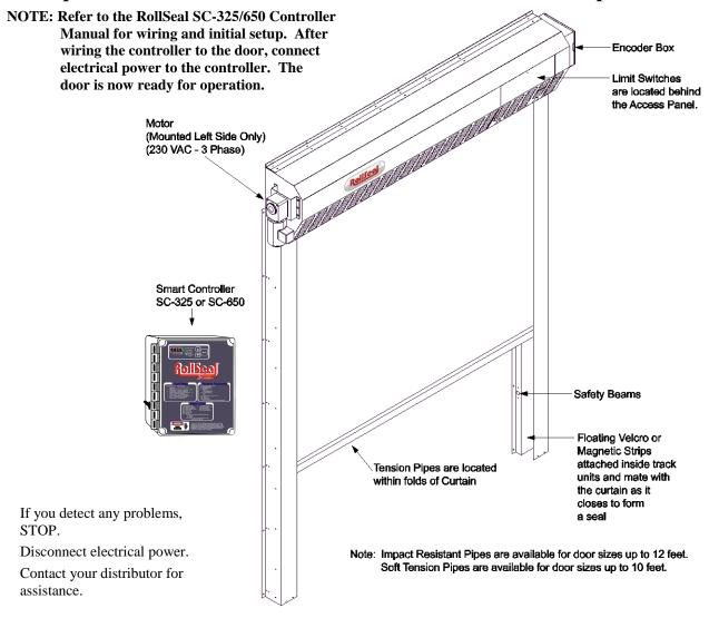
The controller keeps track of the "open" and "closed" positions of the door by means of a mechanical encoder wheel that is located in the encoder box. The controller electronically counts steps as the wheel turns to keep track of the door position. The door seals by means of 'hook & loop' or 'magnetic' strips along the edges of the door curtain and vertical members.
