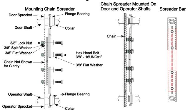
Length of Spreader Bar and chain may vary according to mounting option selected. For motors mounted more than 18" away, the Extended Chain and Spreader Bar must be used. (See Diagram 13A)
