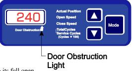
If SWX1:1 is "On", the door will proceed to open to its full open position. If SWX1:1 is "Off", the door will stop and await a command to either continue opening or to close. See **Section 11.1** for the location of SWX1 on the controller PCB 154 circuit board.
