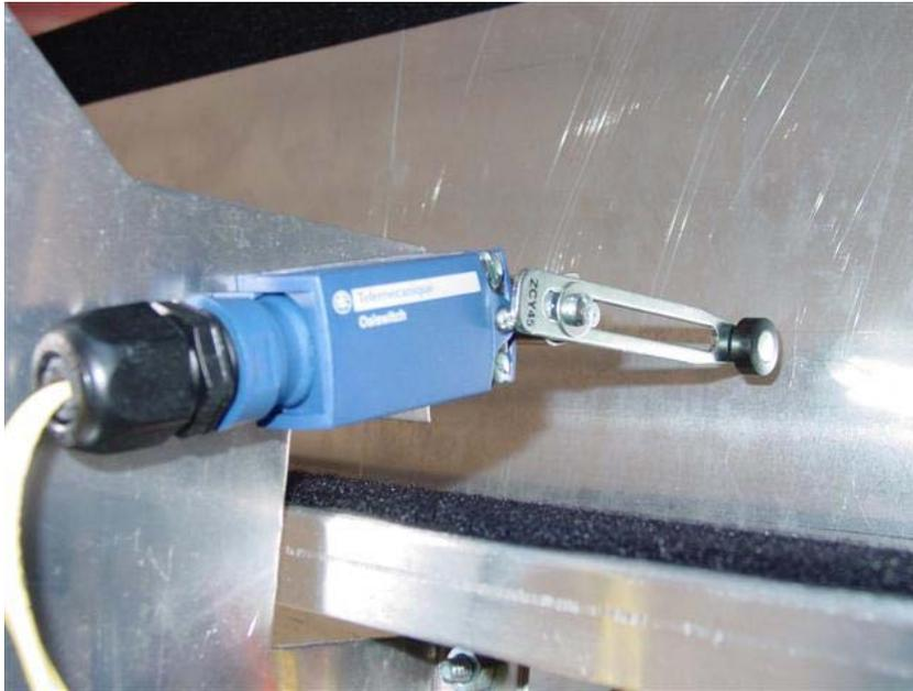
After adjusting the Leading Edge Switch make sure it is positioned downward against the door panel.
