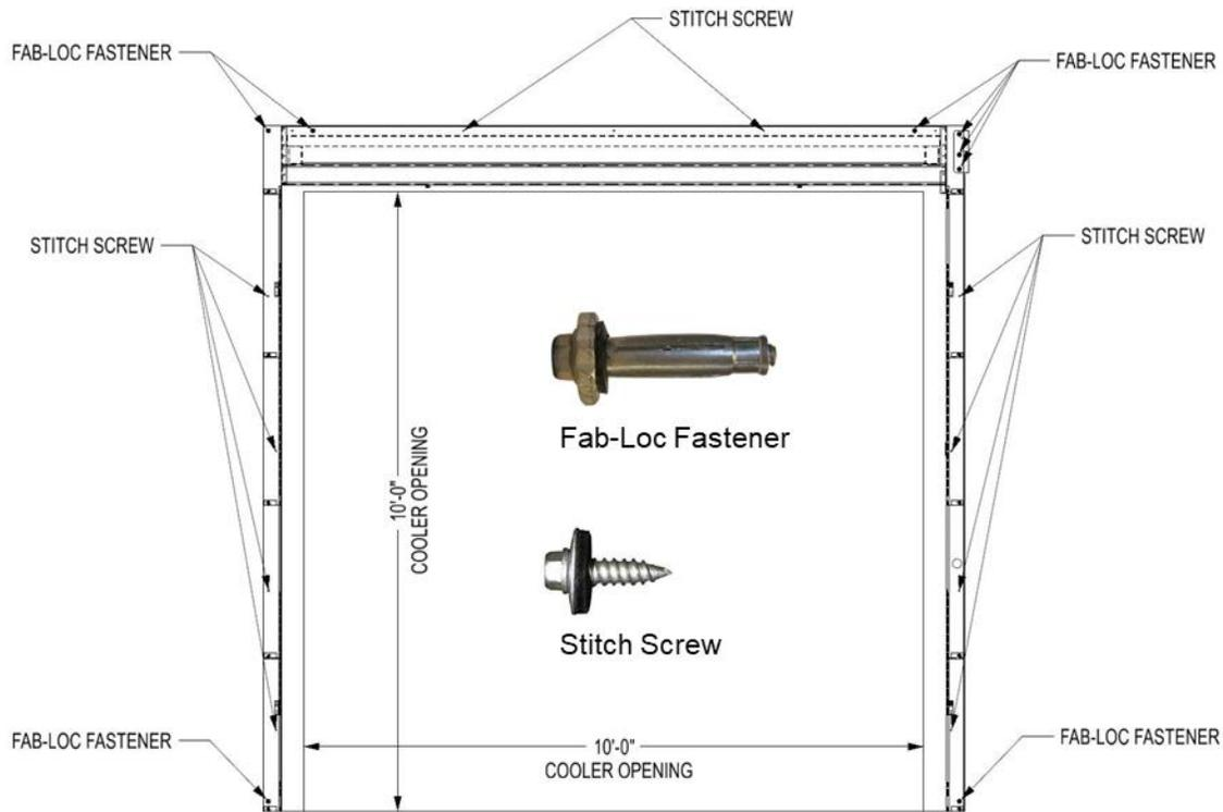
With the left track mounted to the wall, make sure the door is square and plumb across the head and the right track. Mount the right track and back plate with the provided stitch screws.
