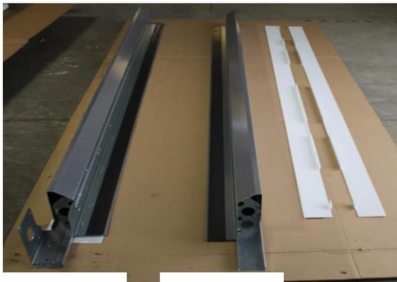
Move the Right and Left track assemblies out so that you can easily access the six phillips head screws on each assembly that hold the cladding to the frame. Remove these screws so that the cladding can be removed from the frame. Put the cladding and screws in the same area as the Front tracks from earlier.
