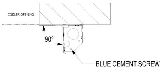
Use a square to ensure that each track is square to the cooler wall face at the bottom. Install a blue cement screw supplied in the hardware kit in the pre-punched hole of the bottom brace on each side.
