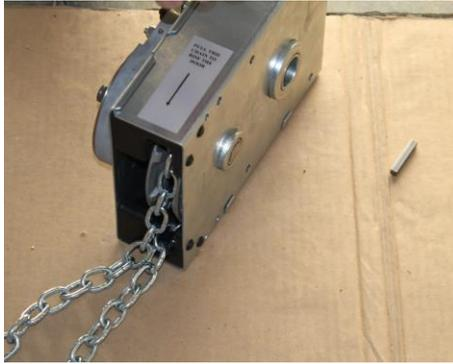
Locate the chain hoist box and open it. The chain hoist comes with the hand chain factory set for this door height, small hardware bag including a  $\frac{1}{4}$ "x $\frac{1}{4}$ "x1" long key and assorted hardware and a chain keeper.
