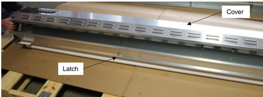
their slots in the frame so that the cover can be removed and set aside with the other cladding until the door frame is installed.
