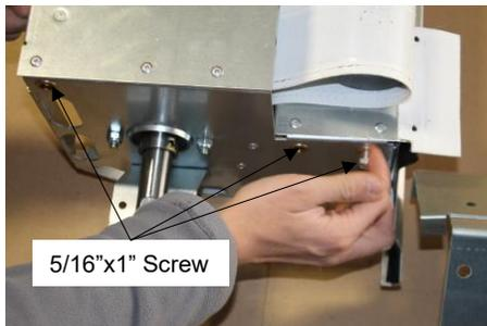
There are three 5/16"x1" bolts on each side of the unit that must be removed so that the track assemblies can be mounted.
