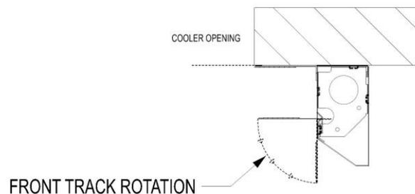
Take the head cover and align the tabs with the slots in the back plate and allow them to drop into place. This will allow the cover to pivot up. Use the “kick stand” mounted on the front bar to hold the cover open.
