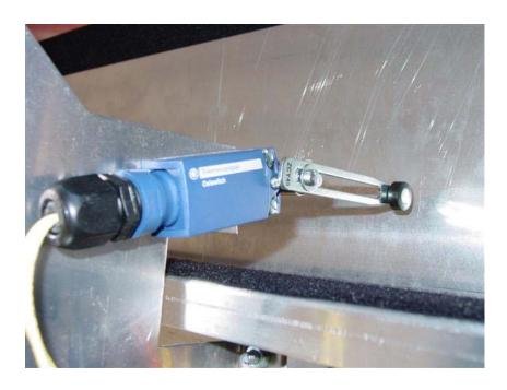
After adjusting the Leading Edge Switch make sure it is positioned downward against the door panel.
