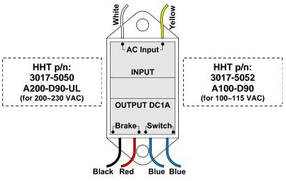
The SC-325 Controllers are factory preset to 115 VAC and the RS-500 Doors are factory prewired to require a 115 VAC power supply.
