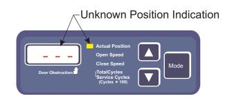
Switch position to the Open Limit position, the Display Indicator will show the Actual Position of the door. This indicates that the door has reset its position and is ready for normal operation.
