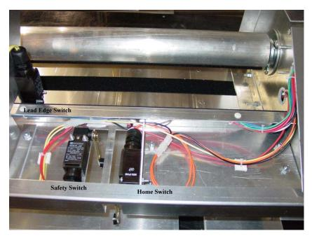
Adjust both the Home Switch and Safety Switch at 90 degrees from its mounted position.
