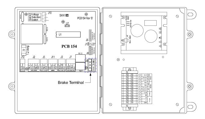
If the Brake Relay is at fault, the door will struggle to operate or could cause the drive board to trip. This situation could create an Error code of EOF1 or ECF1 in the Controller Display.
