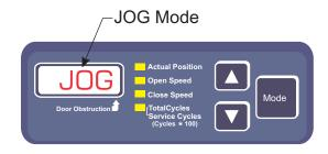
operator must carefully watch the door movement when nearing the full open and full closed positions. To exit the Jog Mode, press and hold the  $Up(\triangle)$  and  $Down(\nabla)$  arrow buttons for at least 5 seconds. The Controller will return to the normal operating mode with the Actual Position shown in the display.
