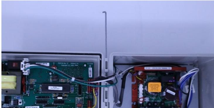
Figure 4: Removing Door Assembly
