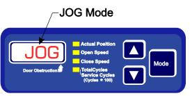
affected by the Home limit switch or the Safety beam. Therefore, the operator must carefully watch the door movement when nearing the full open and full closed positions. To exit the Jog Mode, press and hold the Up ( $\triangle$ ) and **Down** ( $\bigtriangledown$ ) arrow buttons for at least 5 seconds. The controller will return to the normal operating mode with the Actual Position shown in the display.
