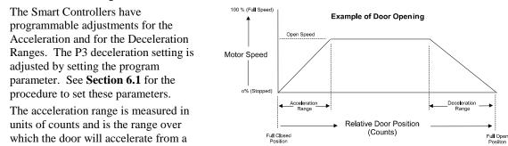
stopped position to the open or close speed. The Deceleration Range is measured in units of counts and is the range over which the door will decelerate from the open or close speed to a stopped position. Typical values for the Acceleration Range are 40 counts and for the Deceleration Range is 80 counts.
